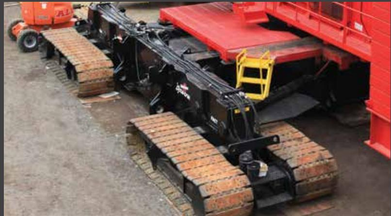
Reduced ground bearing pressure means less time and investment preparing the site to handle the load. This is a distinct advantage at a site like a power plant, where shutdowns for lifting work can cost a power company millions of dollars each day.
