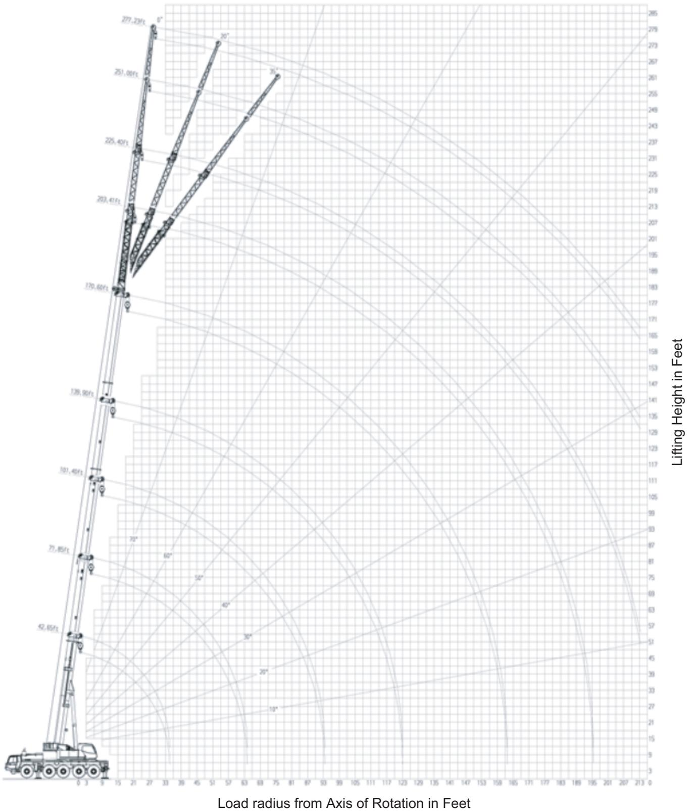
**NOTE:** Boom and jib geometry shown are for unloaded condition and machine standing level on firm supporting surface. Boom deflection and subsequent radius and boom angle change must be accounted for when applying load to hook.
